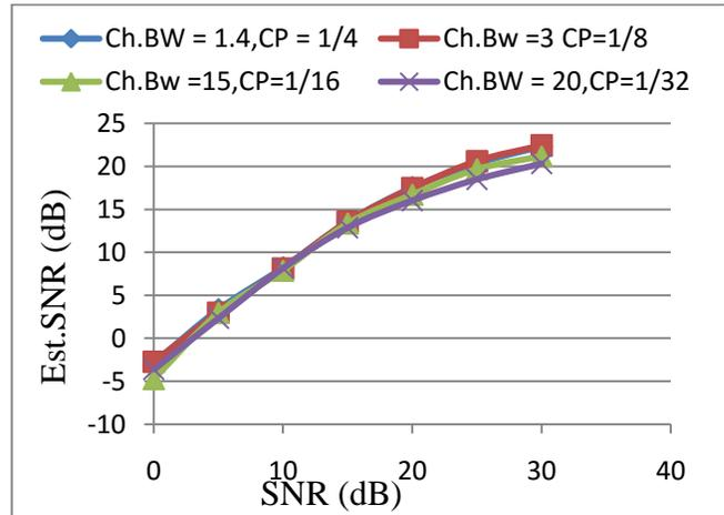
Fig 5.b. Frequency Selective Fading
