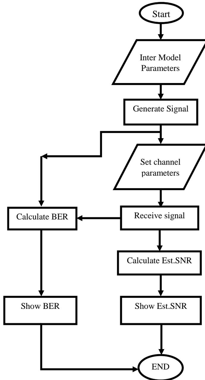
Figure 1: Flowchart for Wireless MAN-OFDM Physical Layer Simulation
