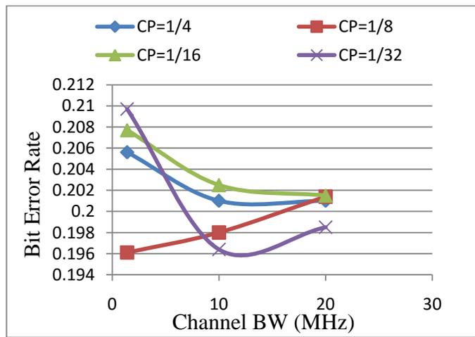
Fig 2.b. Frequency Selective Fading
